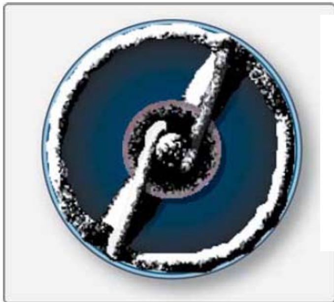
Figure 4-48. Carbon fouled spark plug.
