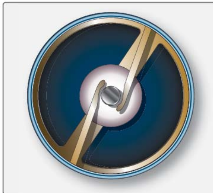
Figure 4-50. Spark plug gap erosion.
