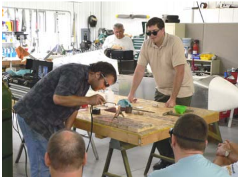
Aaron Novak talked about the welding equipment and material preparation needed for oxy/acetylene welding of aluminum.
