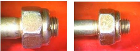
In these photos, with 3 threads showing, you can see there is not much of the threaded portion remaining past the underside of the nut.
