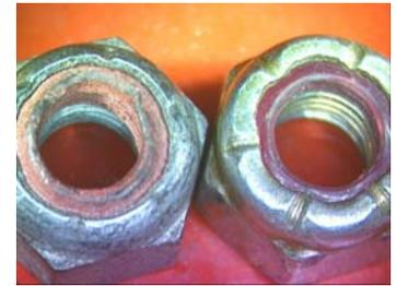
The photos above each contain one elastic (nylon/plastic) lock washer and one fiber type lock washer. The top photo shows unused hardware, the other used hardware. As you can see, close examination reveals the fibrous appearance of the obsolete hardware whereas the newer elastic material has a smooth, plastic appearance.
