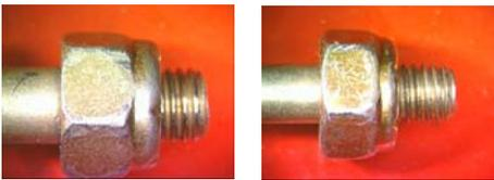
In these photos, the nuts have been threaded on until beginning to contact the unthreaded shank – **this is bad**. You can see there is not a lot of difference between having 3 threads visible, and the nut bottoming out on the shank. Therein lies the problem.
