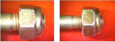
In these photos, we have one thread showing past the self locking feature. You can see that with the AN 3 bolt there is maybe three threads visible on the underside, which amounts to about .094” of usable threaded portion remaining under the nut - which is good. This amount of length can easily be taken up with a couple of washers. One under the bolt head and one under the nut might work nicely.
