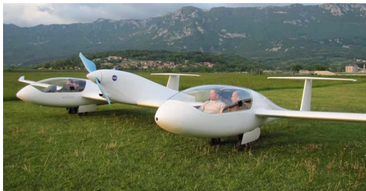
The electric powered Pipistrel Taurus G4. Yes, that is all one airplane.
