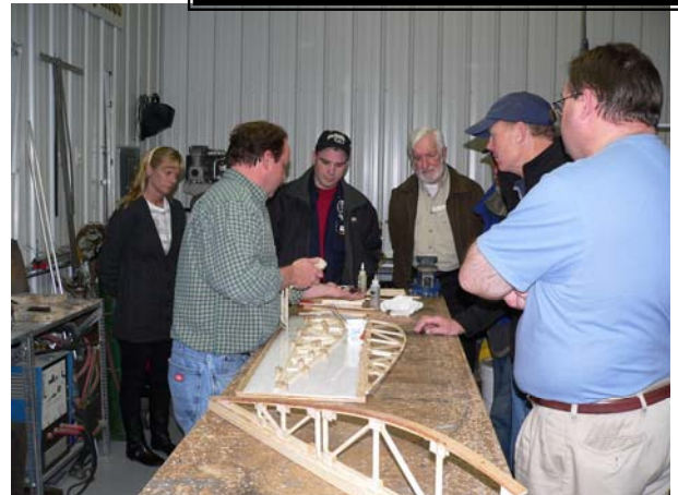
John Egan demonstrates Pietenpol wood rib building techniques.
