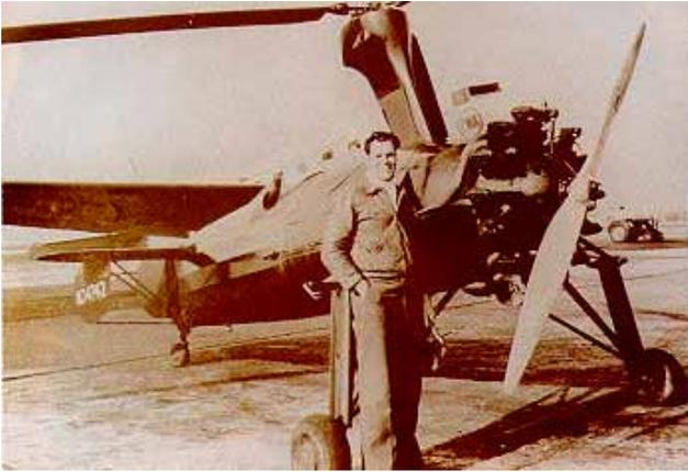
**(COURTESY OF JOHN M. MILLER)** Test pilot John M. Miller with the Kellett KD-1 Autogyro prototype in 1937. All directional control for the KD-1 was provided through a unique tilting rotor head.
