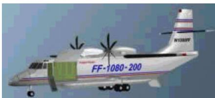
The FF-1080, which has been in development for 13 years will be an all-aluminum, twin engine, high wing, fixed landing gear, non-pressurized, single pilot capable turboprop aircraft with short takeoff and landing capability, specifically designed as a utility air freight transportation system.
